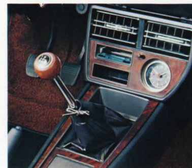
Celica ST standard 4-speed all-synchromesh transmission.
