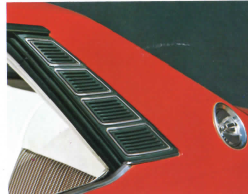
Ventilation system extractor.
